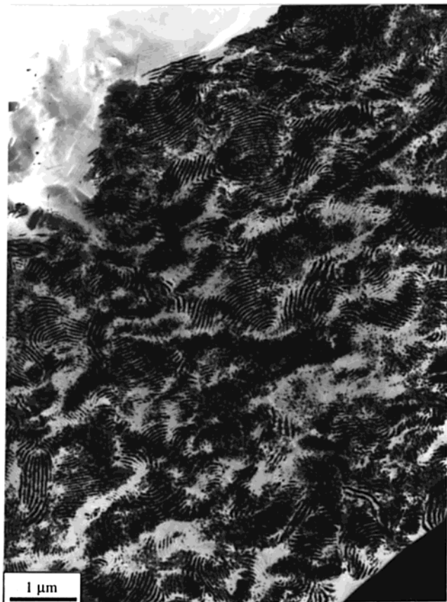
Figure 8. Film treated in “slow-plating” electroless copper bath for 41 h. (Note: lamellae are arranged in randomly oriented grains.)
